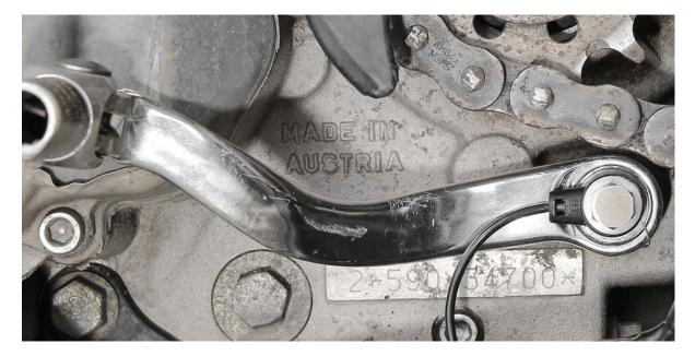
1d. QSE Sensor under the bolt of shift lever (typically on off-road bikes)
