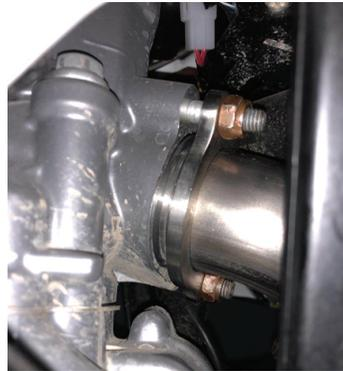
2) Fit the front section of your Tekmo Header into place and do up the engine flange mount bolts lightly so that you can still move the pipe around, making sure that the pipe is seated correctly into the engine exhaust port and the exhaust flange gasket is still in place Diagram A.
