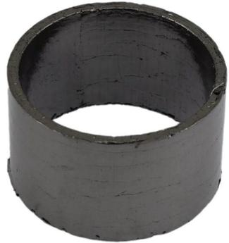
5) Install you rear muffler using the original graphite spacer the muffler mountbolt can be done up tight (If you are replacing your rear muffler at the same time you may need to purchase a graphite spacer from your local Husqvarna dealer depending on what brand rear muffler you buy).
