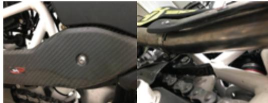
For the **KTM 690** Reinstall the left hand side panel , then install the rear heat shield moving the front bracket into position, install the front heat shield moving the mounting brackets into the correct position then all the pipe clamps for the heat shields can be tightened.
