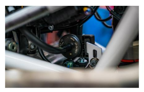
14. Unplug and trace one of the hoses to the canister behind the right fairing and remove it from the frame by pulling it through.
