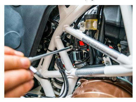
11. Locate the blue colored dongle (pictured in black below) and insert each pin into the harness plug that was plugged into the SAS valve. NOTE: There is no plug that exists for this connection, so this is the method we chose to insert the dongle.
