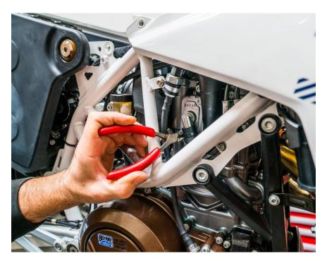
5. Remove the hose that travels from the SAS valve to this plate.
