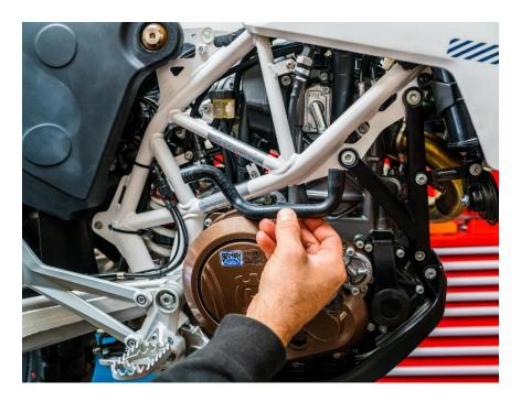
7. (T30 TORX) Remove the two bolts from the SAS plate and remove it. Leave the rubber reed valve in place.
