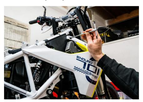
1. (CUTTERS) Locate the SAS valve just beneath the rear brake reservoir (shown below) and cut both zip ties on both hoses.
