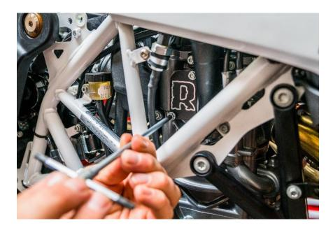
9. (08-13 KTM 690 Only) Unlike the 701, the KTM 690 SAS hose travels from the SAS valve to the top of the head instead of the side of the cylinder. Remove the hose from the port below (arrow) and cap it with the rubber boot and spring clamp included in the 690 specific emissions removal kit.
