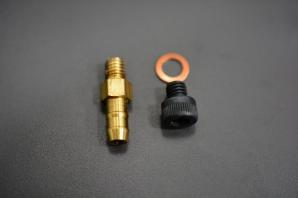
24. (5mm HEX) Replace the nipple with the small 6mm screw and copper washer.
