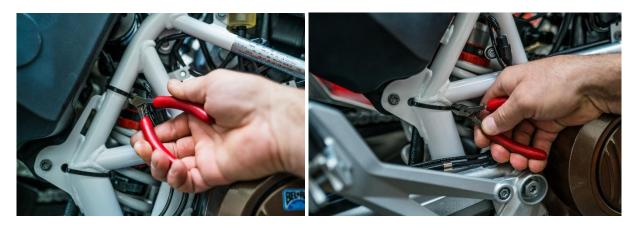
18. CAUTION: FUEL MAY SPLILL FROM THIS CONNECTION! Remove the 'Y' section of the hose and rejoin the fuel tank hose to the other hose on the 'Y' adapter of the same diameter with the included straight barbed fitting. It may help to trim off the ends of the hose where they have expanded to get a tighter fit on the straight barbed connection.
