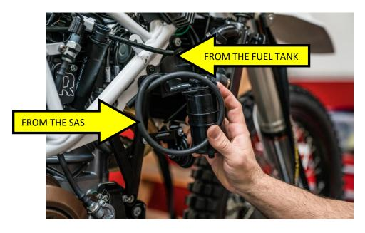
16. (T30 TORX) Remove the mount from the frame.
