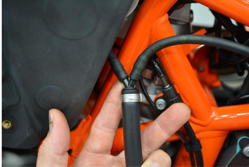
17. **CAUTION: FUEL MAY SPLILL FROM THIS CONNECTION!** Remove the 'Y' section of the hose and rejoin the fuel tank hose to the other hose on the 'Y' adapter of the same diameter with the included straight barbed fitting. It may help to trim off the ends of the hose where they have expanded to get a tighter fit on the straight barbed connection.
