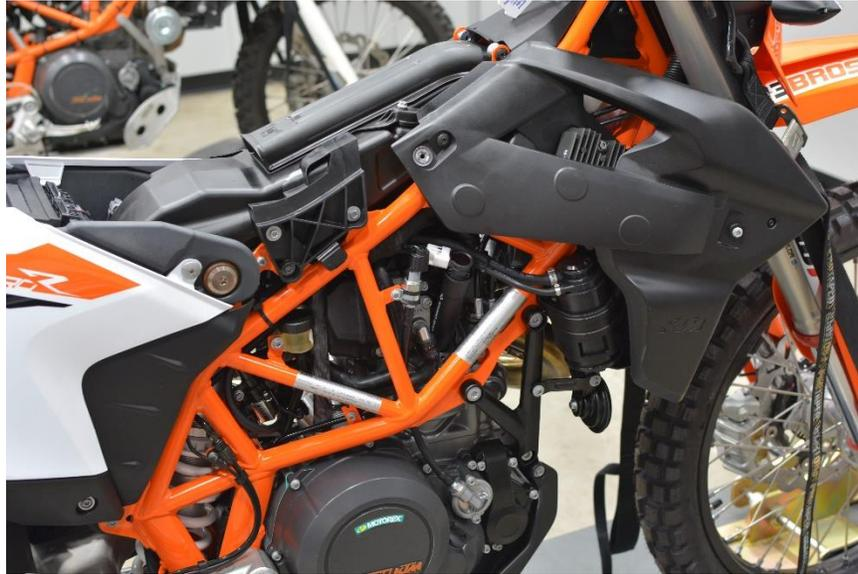
2. (T30/20 TORX) Remove the right-side inner panel. The GREEN circle notes a pin that can be released by hand.
