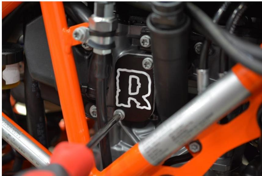
7. (T30 TORX) Remove the SAS valve from the frame and unplug the electrical connection.
