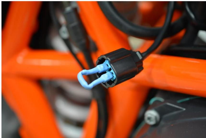
9. (HEAT GUN) Use the large glue lined heat shrink to create a watertight seal around the plug. To make this step easily reversible you may just heat the ends so that the glue is tacky and seal them without shrinking the entire part. **CAUTION: Use protection to avoid burning your fingers.** This will be zip tied at line 19.
