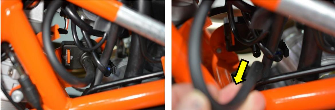
12. Pull the thicker of the two lines at the canister through the frame and out. You may have to rotate the outer coil stick to allow the line to pass through behind it.
