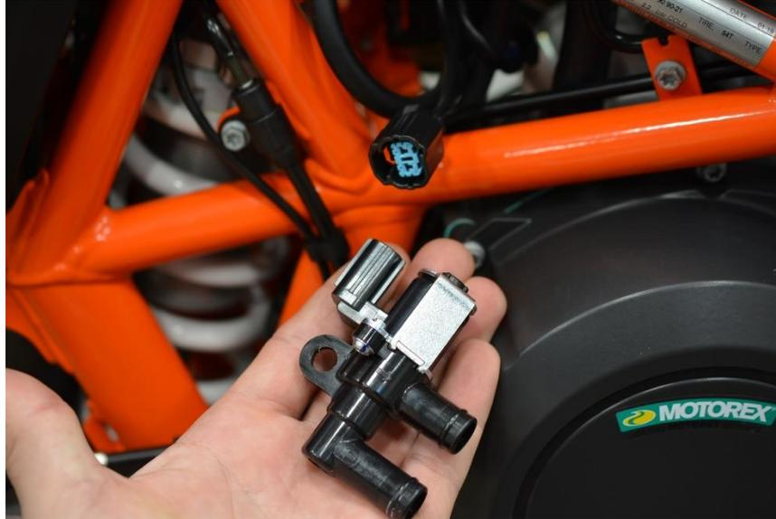
8. Locate the blue colored dongle and insert each pin into the harness plug that was plugged into the SAS valve. NOTE: There is no plug that exists for this connection, so this is the method we chose to insert the dongle.
