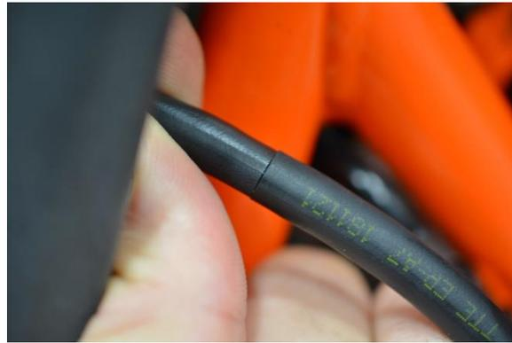
18. Route the newly joined line through the frame and towards the ground. Zip tie the line to the same tabs that recently held the thicker tube and some electrical wires and trim to length.
