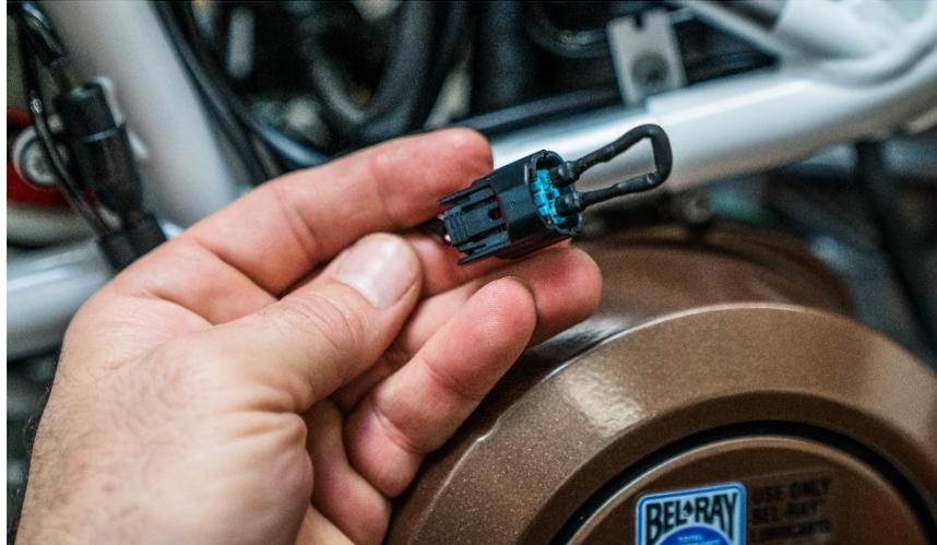
12. Using the large glue lined heat shrink to create a water tight seal around the plug. **CAUTION: Use gloves to avoid burning your fingers.**
