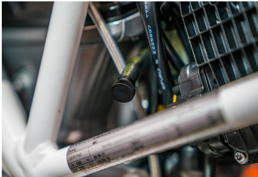
25. Choice #2: Trace the line to the head and remove the brass nipple with a deep 8mm socket.
