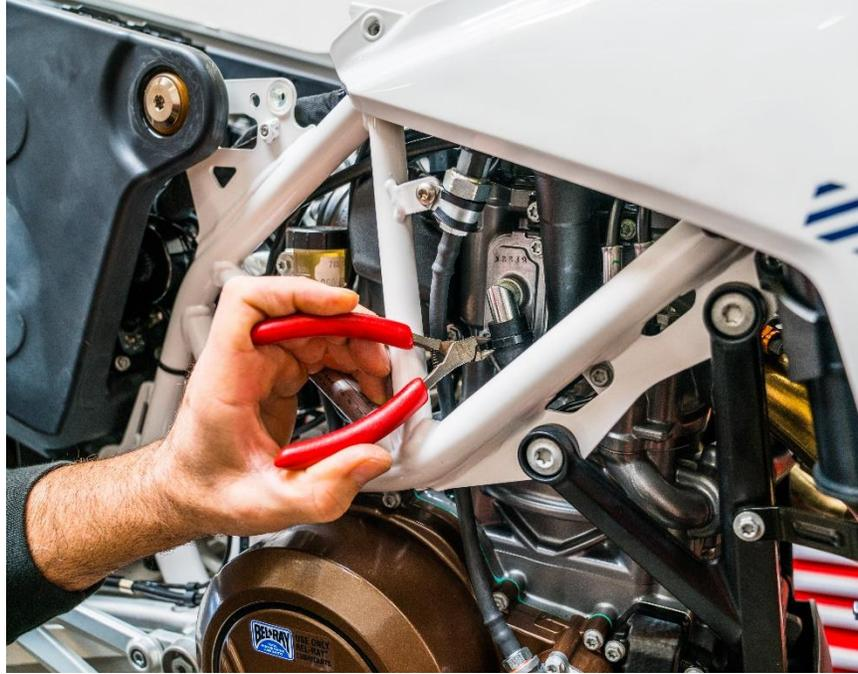
6. Remove the hose that travels from the SAS valve to this plate.
