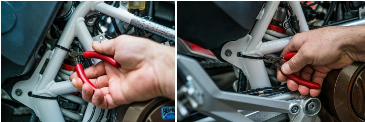
19. Remove the 'Y' section of the hose and rejoin the fuel tank hose to the other hose on the 'Y' adapter of the same diameter with the straight barbed fitting.
