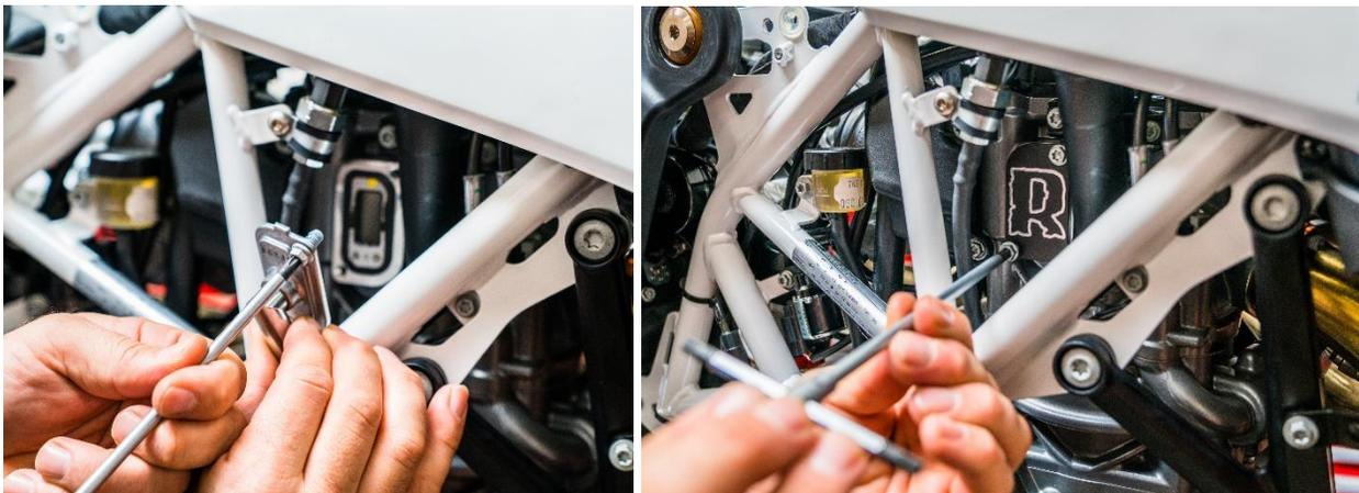
9. (08-13 KTM 690 Only) Unlike the 701, the KTM 690 SAS hose travels from the SAS valve to the top of the head instead of the side of the cylinder. Remove the hose from the port below (arrow) and cap it with the rubber boot and spring clamp included in the 690 specific emissions removal kit.
