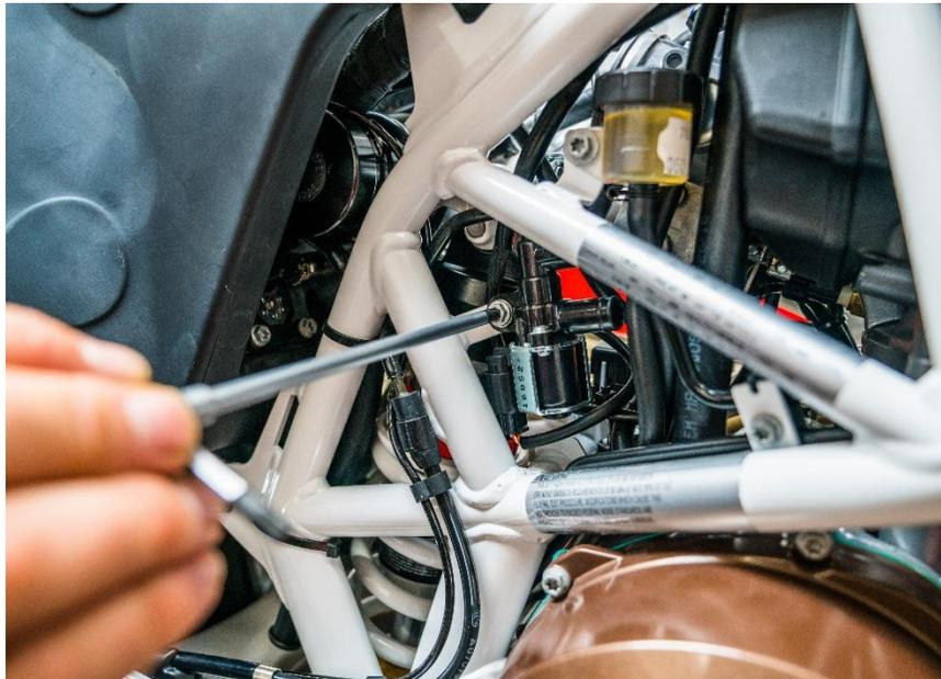
11. Locate the blue colored dongle (pictured in black below) and insert each pin into the harness plug that was plugged into the SAS valve. NOTE: There is no plug in existence for this connection so this is the method we chose to insert the dongle.
