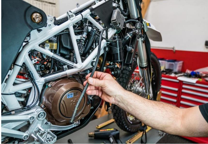
15. Identify the hose traveling from the rear fuel tank to the canister and unplug it from the canister.
